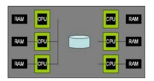
The underlying storage area network might use any of a number of block-level protocols, including SCSI, <u>iSCSI</u>, <u>HyperSCSI</u>, ATA over Ethernet (AoE), Fibre Channel, and <u>InfiniBand</u>.
